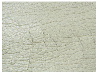
Fractures extend all over the seating area. Impossible to repair.
