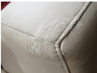
The surface starts peeling off. Impossible to repair.
