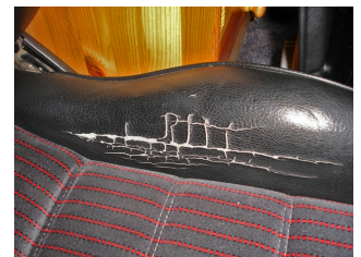
Driver seat: Entire surface is brittle. Should be re-trimmed.
